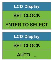
Use left ◀ and right ▶ arrow key to change from AUTO to MANUAL Date/Time set up.
