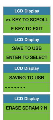
When the system has finished uploading the data to the USB memory stick the LCD display will prompt you to erase the SDRAM. Once you have made your selection  $\mathbf{Y}$  or  $\mathbf{N}$  the system will automatically bring you back to the main screen in the supervisor menu.
