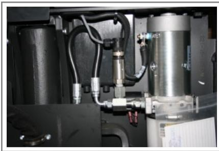
The pressure transducer must be installed in the lifting hydraulic line **between the lift control valve and lift cylinder**. Mount a T-piece in hydraulic line for the installation of the pressure transducer.
