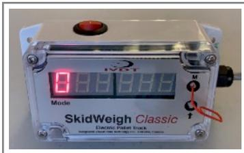
\***Activate and hold lift control switch until lift pump motor stops automatically.** The LED Display will go blank and within few seconds will show “0” digit in furthest right digit display
