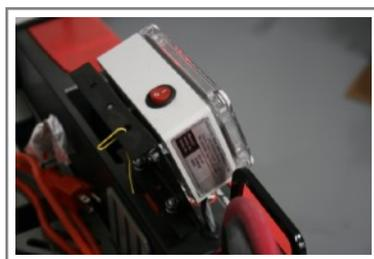
Use the mounting bracket with the anti vibration mounts and fasten the digital indicator to the vehicle dashboard, or any other convenient place on the electric pallet truck body. There are many examples of mounting locations that will depend on the vehicle model. However, additional mounting items such as a flat brackets may be needed to help secure the unit.
