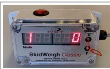
\*The algorithm software controls lifted forks travel, will calculate and store the value of empty forks being lifted.
