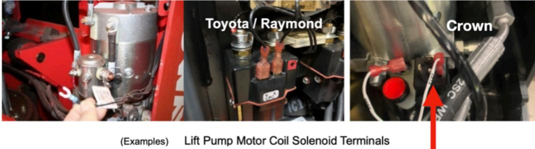
Disconnect one wire from solenoid coil terminals, **positive** or **negative** side. Splice two wires from the indicator in **series with disconnected wire and coil terminal**.
