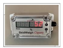
The SC4 SkidWeigh Classic system operational principal is based on the hydraulic pressure transducer mounted in the vehicle lifting hydraulic circuit. The patented algorithm will initiate the measurement cycle every time a load is lifted. The increase in pressure is converted in an electronic signal at the sample rate of 16000 readings per measurement cycle, updated every second which is converted into a capacity load readout shown in percentage of the vehicle maximum load lifting capacity.
