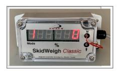
Wait few seconds, LED display will go blank for \*few seconds and will show in **Mode** digit number **1** and default value of "**0**" in furthest right digit display.
