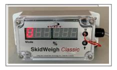
When LED display is showing "0" in **Mode** digit, lift the empty forks (or attachment such as longer forks, clamp, etc) just above the ground.
