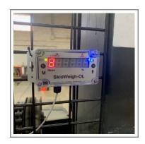
After you have connected two wires to the vehicle power and pressure transducer cable you can "quickly" check the system operation.
