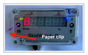
To initiate calibration press the "**M**" button (use a paper clip) and hold it down for approx. 5 seconds.
