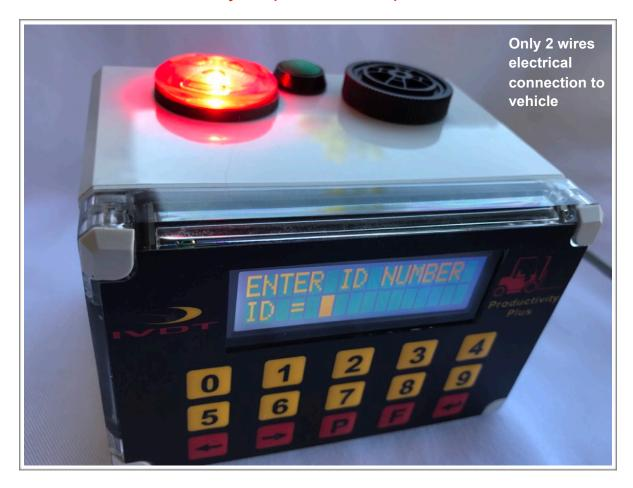
The **OSC3-LT** is a simple comprehensive unit designed to provide single lift truck or small fleet with the ability to control that only certified operators are allowed access to the lift trucks and ensure that prior to shift use a safety check is done. Operating as a stand-alone unit the OSC3-LT will consistently and accurately provide management with permanent record of daily OSHA safety inspection compliance.
