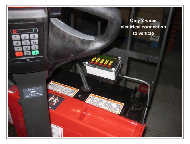
The **OSC1-EP** is a simple comprehensive unit designed to provide single electric pallet truck or small fleet with the ability to control that only certified operators are allowed access to the lift trucks and ensure that prior to shift use a safety check is done.
