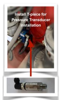
Before mounting the pressure transducer in the hydraulic lift circuit make sure that system is pressure free.
