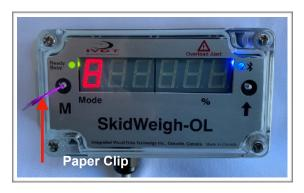
After approximately five-seconds the Mode LED display digit will change from **Mode 8** to **Mode 0**. System is ready for automatic zeroing
