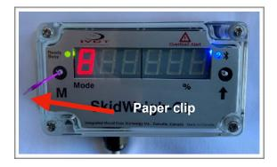
To initiate calibration press the "**M**" button (use a paper clip) and hold it down for approx. 5 seconds.
