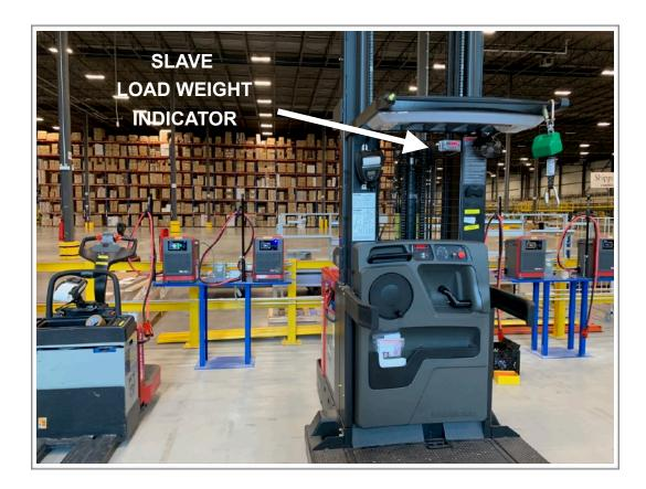
Turn on vehicle power switch. With forks lowered to ground SLAVE indicator will show software version and Mode 8 will be shown on LED display.
