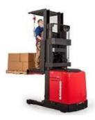
\* Drive your vehicle into the skid load with known weight at load centre of 24" and lift the load to the highest operational forks height.
