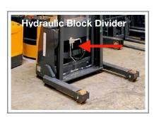
Before mounting the pressure transducer in the hydraulic lift circuit make sure that system is pressure free.
