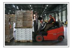
3. Lift loaded forks just above the ground and within few seconds LED display will show weight.
