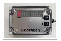
Lower the load to the ground. System will go automatically into operational mode. System is ready to be used. Mode digit will display number **8**.
