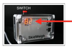
Weighing Channel 2 The Mode 82 digit will be show on LED display.
