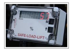
LED display readout of lifted load shown in % of maximum vehicle lifting capacity will be updated every second.
