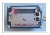
When LED display is showing "0" in Mode digit, lift the empty forks just above the ground to automatically calibrate zero value for empty forks being lifted.
