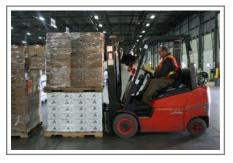
3. Lift loaded forks just above the ground and within few seconds LED display will show weight.
