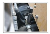
normal operation. Pressure transducer has 1/4"-18 NPT male thread. Use thread seal to ensure tight fit.
