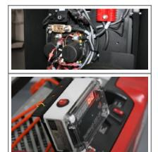
Consult vehicle CANbus controller wiring diagram or contact the OEM for proper interface of two black wires to control lift pump motor travel
