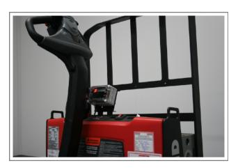
Use the mounting bracket with the anti vibration mount and fasten digital indicator on the vehicle dashboard, load backrest or any other convenient place on the electric pallet truck dashboard body There are many examples of mounting locations that will depend on the vehicle model. However, additional mounting items such as a flat brackets may be needed to help secure the unit.
