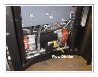
The pressure transducer must be installed in the hydraulic lift line between the lift control valve and lift cylinder(s). In some cases you can install the pressure transducer in the flow divider, drilling and tapping for 1/4"-18 NPT male in spare plug or in the body of the flow divider. Also, you can drill and tap on any "larger elbow" that might be available in the hydraulic lift circuit found in vehicles with larger hoses to accommodate larger vehicle lifting capacities.
