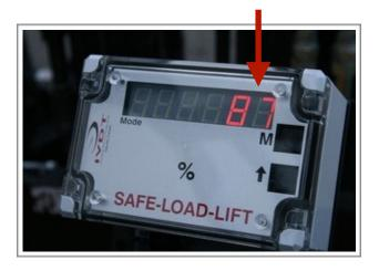
\* To deactivate overload alert operator must lower the loaded forks to the ground.
