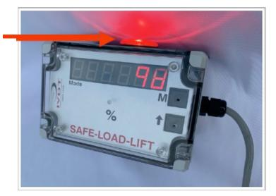
Overload Audio / Visual Alert at 98% Load Capacity
