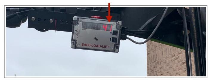
\* If the lifted load is more than preset overload value for the application the overload value will be shown on LED display and (Visual, Audio or both warning) will be activated.
