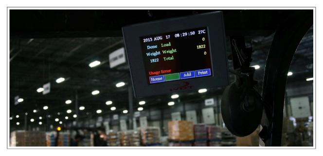
Lift Truck Onboard Check Weighing Scale 5.7" Touch Screen
