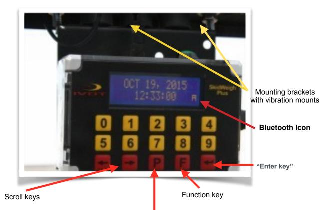
With LCD showing load weight press "P" key and barcode label with data will be provided
