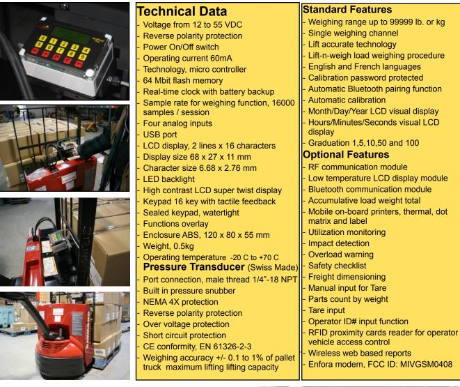
High contrast LCD display with LED backlight, super twist, 2 lines x 16 characters
