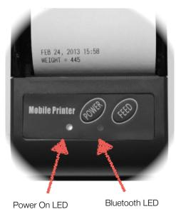
SkidWeigh system with accumulative load weight total with Onboard Printer (Bluetooth)
