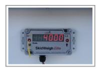
LED display will go blank and within few seconds LED display will show the value of calibrated "Known load weight of 4000"
