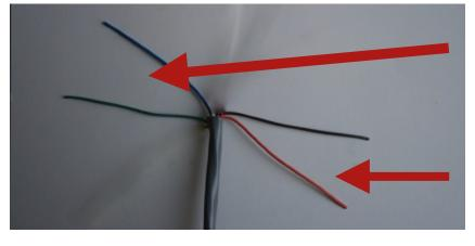
Use two wires **BLUE** and **GREEN** and connect them is series with vehicle seat switch wire **Normally Open Contacts**
