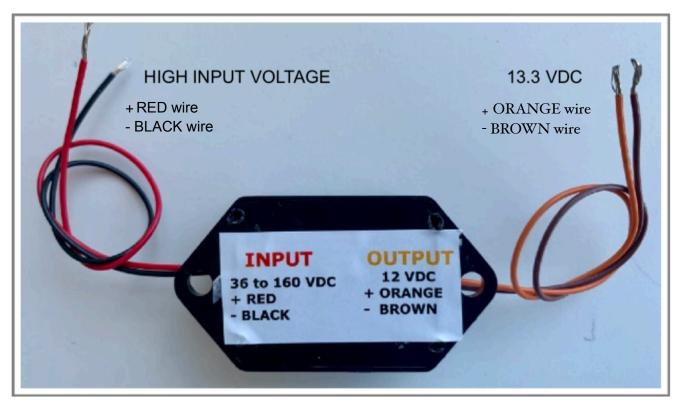
The VC160 series DC/DC converter is designed for material handling vehicles with an extra wide continuous input voltage range of 36-160 VDC, making it suitable for 48 to120 V DC vehicles electrical systems. The high efficiency permits an ambient temperature range from - 40 C to +85 C without derating, forced cooling or the need for heatsinks.
