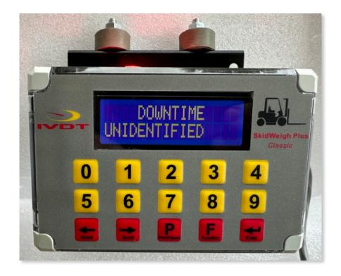
Forklift weighing scales including automatic unidentified operational downtime events, pre-shift safety check, keypad operator access control, multiple colour alert lights and USB port
