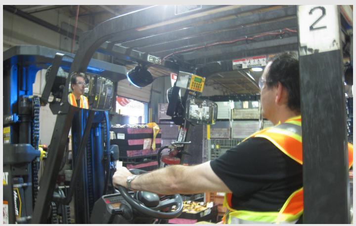
Forklift operators perform at higher utilization factor level when they know performance status is visually shown to them in real time and is being recorded. The automatic **\*true operational idling times** trend reports will show when key KPI variable is outside the target range for each operator. Automated e-mail notifications, LAN web page allow immediate response to actual operational status for each operator that can be addressed, identify and corrective action can be taken.
