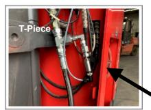
Make sure that that installed pressure transducer will not touch any moving parts or assembly of the vehicle while in normal operation.
