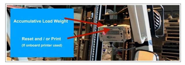
**Note:** If onboard Bluetooth printer connected by pressing "**Red**" button the printer will provide individual or all individual and total accumulative load weight ticket
