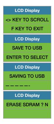
When the system has finished uploading the data to the USB memory stick the LCD display will prompt you to erase the SDRAM, all files contained on the UTX SkidWeigh Plus.
