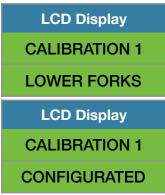
As soon the loaded forks are lowered to the ground the LCD display will show date / time . System check weighing function calibration is completed.
