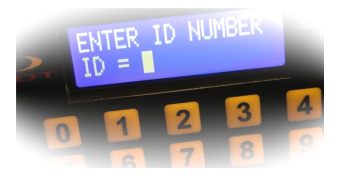
To enter into the **Administration Menu**, press **F** key and than press **9** key. Input password **521.** Use **left and right arrow keys to scroll for functions** that might apply for your system configuration.
