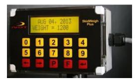
This load weight will be shown on LCD display until next time the forks are lowered to ground.
