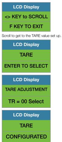
To reset or change TARE value press **F 0** key and set to 0 to reset current TARE value or input new TARE value and press **"Enter key"** ← .
