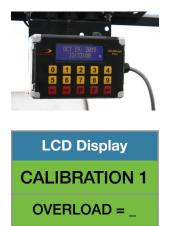
Input the overload value (as of example 5500 ) and press "Enter key" ←.
