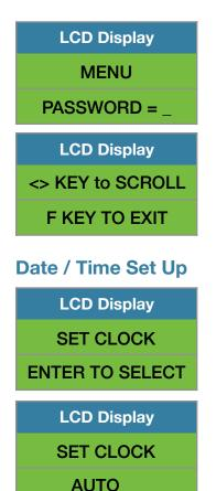
Use left ◀ and right ► arrow key (*bottom left side of the keypad*) to change from AUTO to MANUAL date/time set up.
