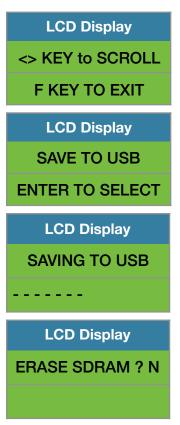
When the system has finished uploading the data to the USB memory stick the LCD display will prompt you to erase the SDRAM, all files contained on the SKidWeigh Plus ED3-UT-IM. Once you have made your selection  $\mathbf{Y}$  or  $\mathbf{N}$  the system will automatically bring you back to the main screen in the supervisor menu.
