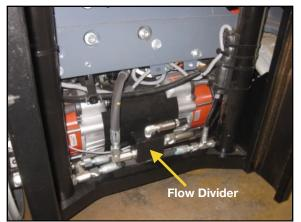
The pressure transducer must be installed in the hydraulic lift line **between the lift control valve and lift cylinder(s).** In some cases you can install the pressure transducer in the flow divider, drilling and tapping for 1/4"-18 NPT male in spare plug or in the body of the flow divider. Also, you can drill and tap on any "larger elbow" that might be available in the hydraulic lift circuit found in vehicles with larger hoses to accommodate larger vehicle lifting capacities.
