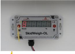
After 5 seconds the Mode display digit will change from number 8 to 0. (System is ready for automatic zeroing of the scale function)
