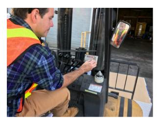
Using the "M" and "Up Arrow" buttons enter the overload weight value for your application similar to the process when calibrating the system with a load weight except the MODE 7 digit remains throughout this operation. Once the last digit has been entered MODE 7 will disappear.
