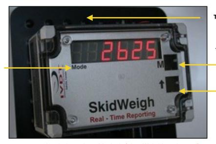
Two Weighing Channel Switch
